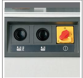
Push buttons allow, that the automatic clamp can be moved up and down independent of blade movement.
