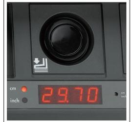
**NEW:** Precise backgauge positioning with the hand crank is very easy due to the digital measurement readout, which can be switched over from cm to inch.
