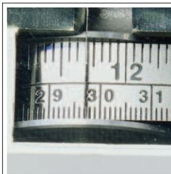
The precise measuring scale (mm/inches) for the backgauge positioning can be read easily and is located on the front table.
