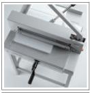
Transparent safety guards made from unbreakable Lexan® on front and rear table: The hinged
