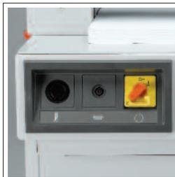
The numerous features of SCS (Safety Cutting System) include a main switch, a true two-hand operation as well as an electric lock with key.
