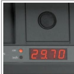
Precise backgauge positioning with the hand crank is very easy due to the digital measurement readout, which can be switched over from cm to inch.
