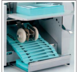
Stream delivery paper ejection system with conveyor belt and adjustable ejection roller
