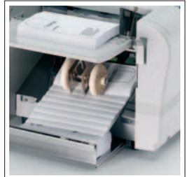
Stream delivery paper ejection system with conveyor belts, ejection roller and adjustable paper tray.
